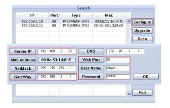
Step3: Select the IP address you want to configure, and click "Configure" to show the IP setting page, and change the IP address, gateway and port number.
