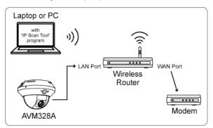
→ Devices connected with a RJ45 network cable
