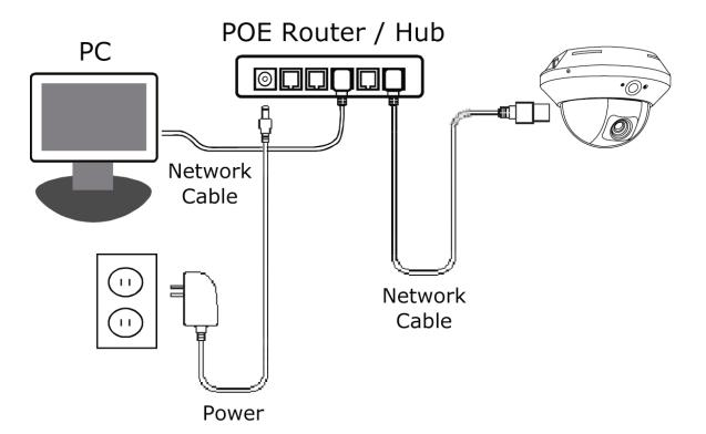
■ When your router / hub doesn't support POE connection (An optional POE connected required)
